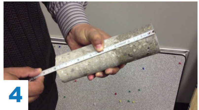
DRIED AFTER 4 MINUTES SHOWS DEPTH OF PENETRATION BY WET SECTION
