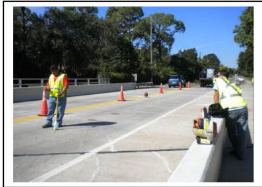
Figures 2 and 3: Half-cell corrosion potential testing (left) and treating bridge deck with SCP (right)
